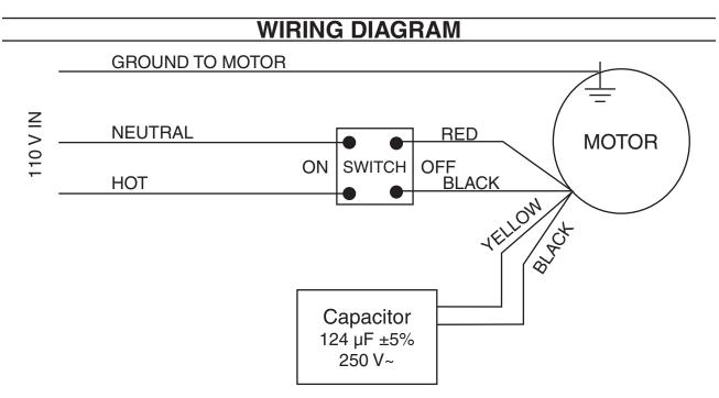
Capacitor is not Polarity - Specific
